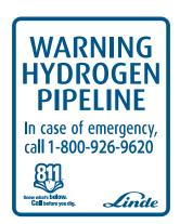
Pipeline markers have been placed at pipeline crossings of public roads, railroads, navigable waterways and other locations to mark the presence of underground pipelines. Linde pipeline markers are generally white rectangular signs with blue or green lettering. These markers display the material transported in the pipeline and the phone number to call in the event of an emergency or if a leak is suspected. You should be
